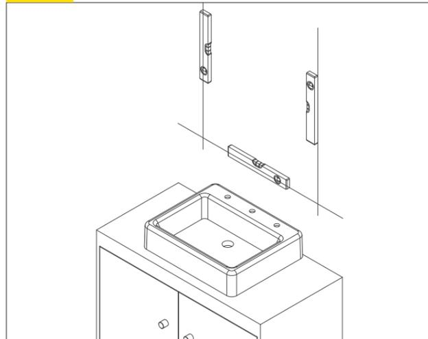
With your level plumb, mark a vertical line on the wall where the edge of the mirror is to be installed.
