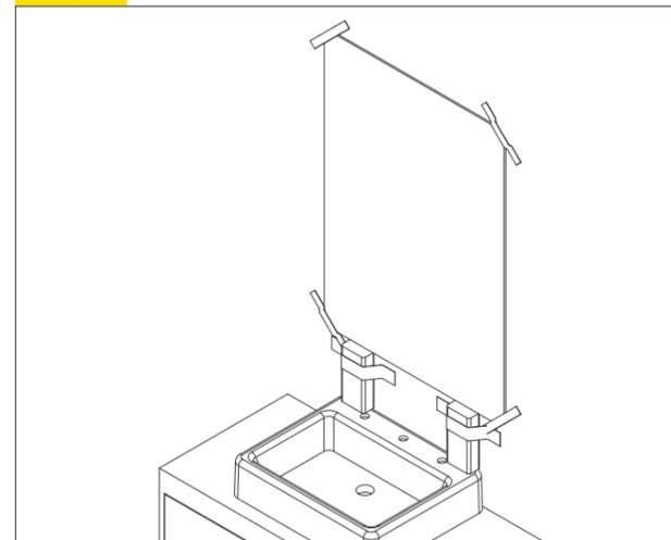
Apply tape to each corner of mirror to ensure mirror does not move.
