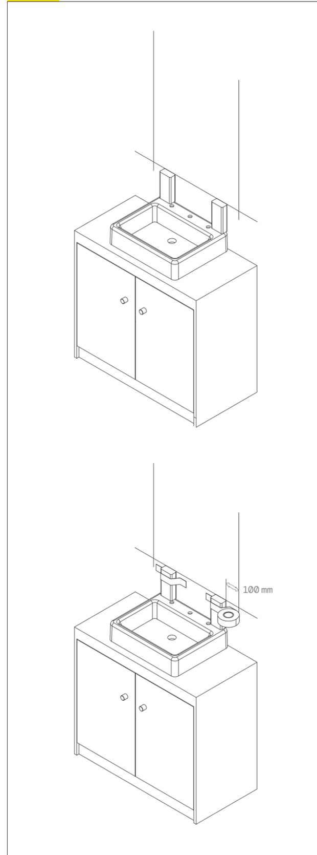
Tape packers to wall approx 100 mm in from each end of the mirror location.
