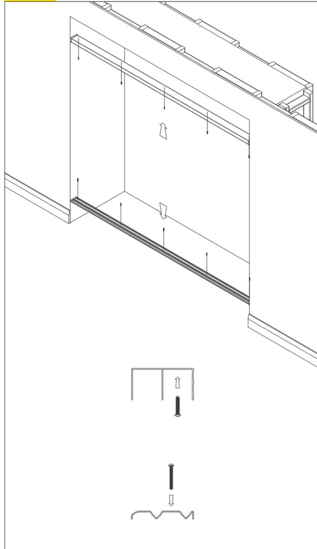
Fix top track flush with front of opening (jamb). Fix bottom track to floor.
