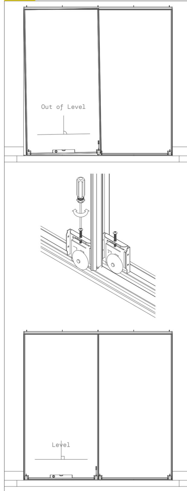
Adjust wheels using Phillips head screwdriver, winding up or down until door is plumb against side jamb.
